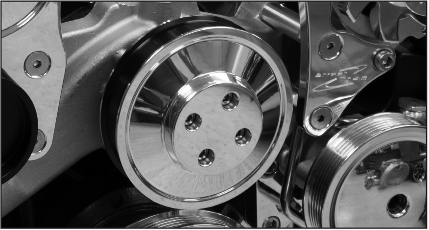
Figure 11: Install Water Pump Pulley
