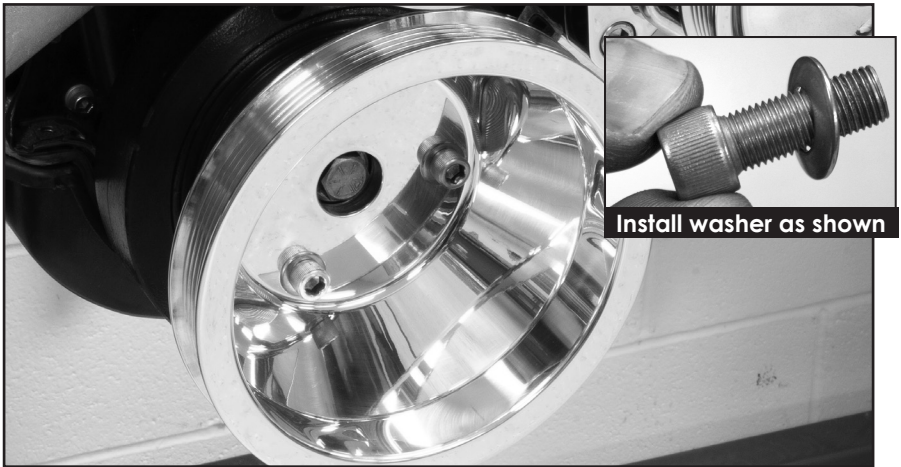
Figure 12: Install Crank Pulley
