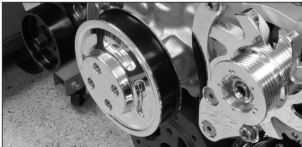
Figure 11: Install Water Pump Pulley
